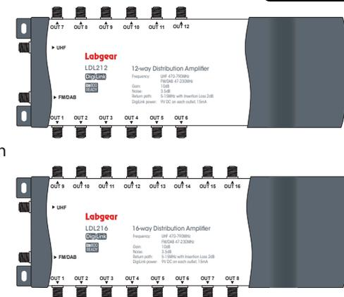
Separate inputs are provided for UHF TV (470-790 MHz) and for FM/DAB (88-230 MHz). Remote capability is provided over a 5-15 MHz RF return path.
