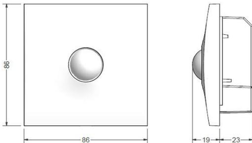
The PDS-PRM presence detector switches are designed to provide automatic control of lighting, heating or ventilation loads. They detect movement using a PIR sensor and turn the load on. When an area is no longer occupied the load will switch off after an adjustable time out period.
