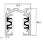
Live conductor Neutral conductor Lip ensures adaptor can only fit when correctly aligned
