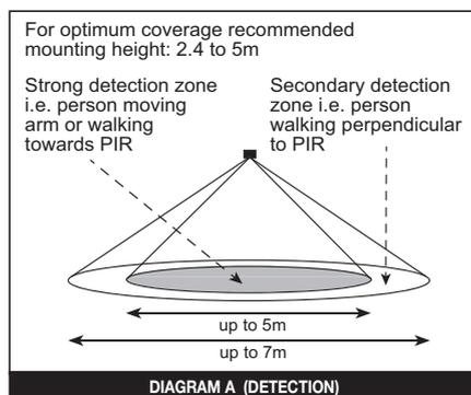
Upon detecting movement, if the ambient light is dark enough, the CESF PIR will switch the load on. The ambient threshold can be set by the user to between approximately 30 lux and 1000 lux and maximum (photocell inactive) at the PIR via the LUX adjuster (diagram B).
