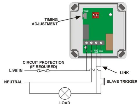
Diagram 2 Wiring for three wire switching circuits
