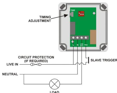
Diagram 1 Standard Wiring
