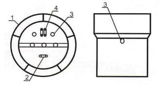
1. Housing; 2. Clip for power supply cords; 3. Holes for power supply cords; 4. Clamp terminal.
