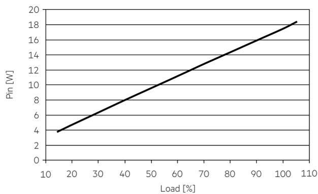
4.1.6 Phase cut dimming curve (depends dimmer)
