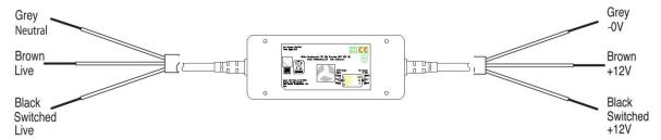
The power supply unit does not require dismantling and should be installed by a qualified electrician to BS7161:2008 (IEEE wiring standards 17<sup>th</sup> Edition). The maximum length of wire between the power supply and the fan should not exceed 5m using 1.5mm<sup>2</sup> wire.
