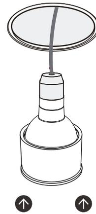
Fit by simply pushing the fixture into the ceiling making sure it is axially aligned.
