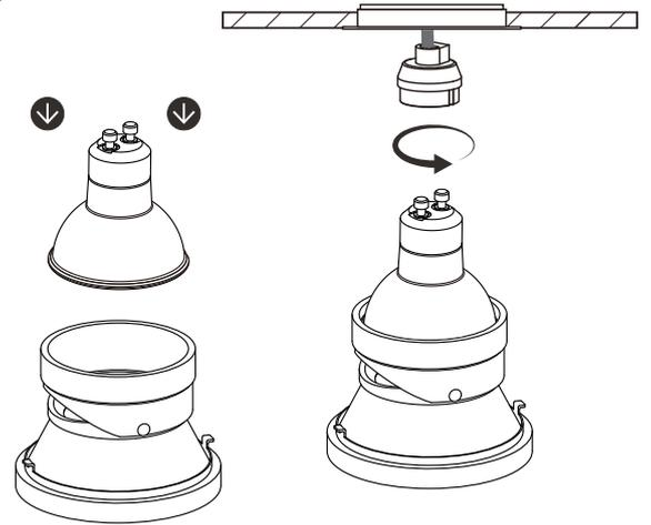
Fit the LED bulb into the fixture, then twist and connect your LED bulb. Finally fit the inner fixture making sure the tilt angle / direction is set as per step 3.
