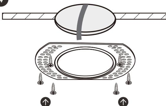
Fit the plaster fixture in the orientation as per step 3. Secure in place with a minimum of 6 screws.
