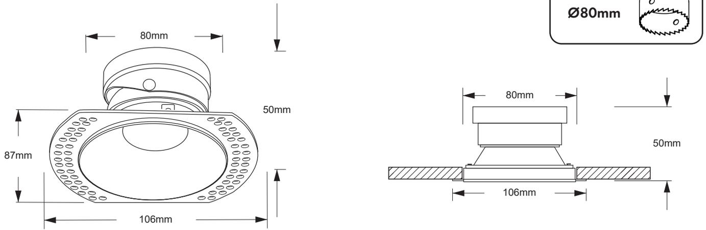
When installed in conjunction with our 'Insulation bracket' (Sold Separately) this product is suitable for coverage by thermal and acoustic insulation e.g. loft insulation. Not suitable for blown insulation. Please ensure a max wattage of 7W when covering with insulation and utilising the insulation bracket.
