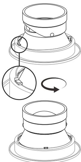
It is advised to test the tilt angle / direction by fitting the fixture together at this stage. Fit the fixture together by aligning the tabs and then rotating the inner cup until tight.
