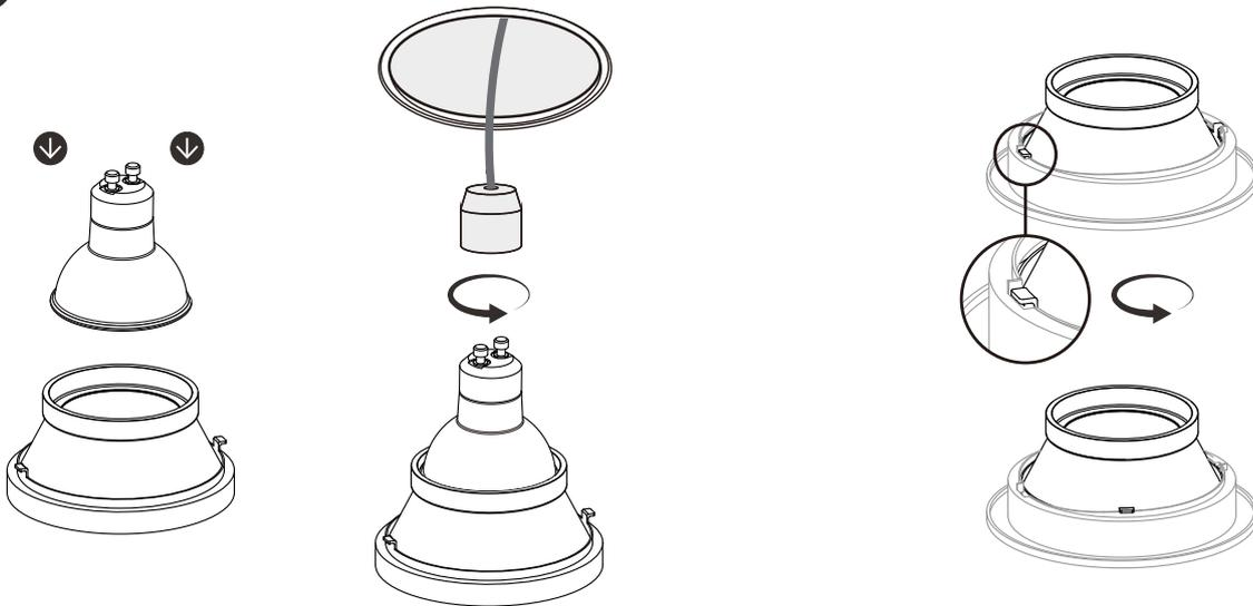
Fit the LED bulb into the fixture, then twist and connect your LED bulb.
