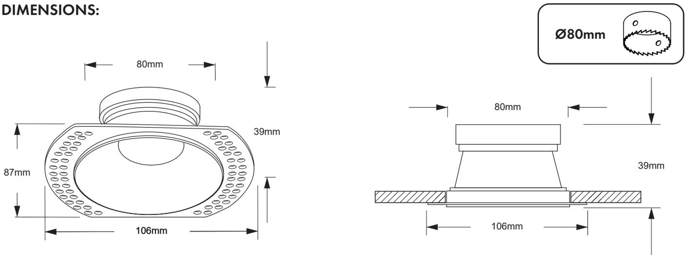
When installed in conjunction with our 'Insulation bracket' (Sold Separately) this product is suitable for coverage by thermal and acoustic insulation e.g. loft insulation. Not suitable for blown insulation. Please ensure a max wattage of 7W when covering with insulation and utilising the insulation bracket.
