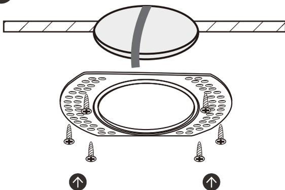
Screw a minimum of 6 screws to the fixture to keep it in place.
