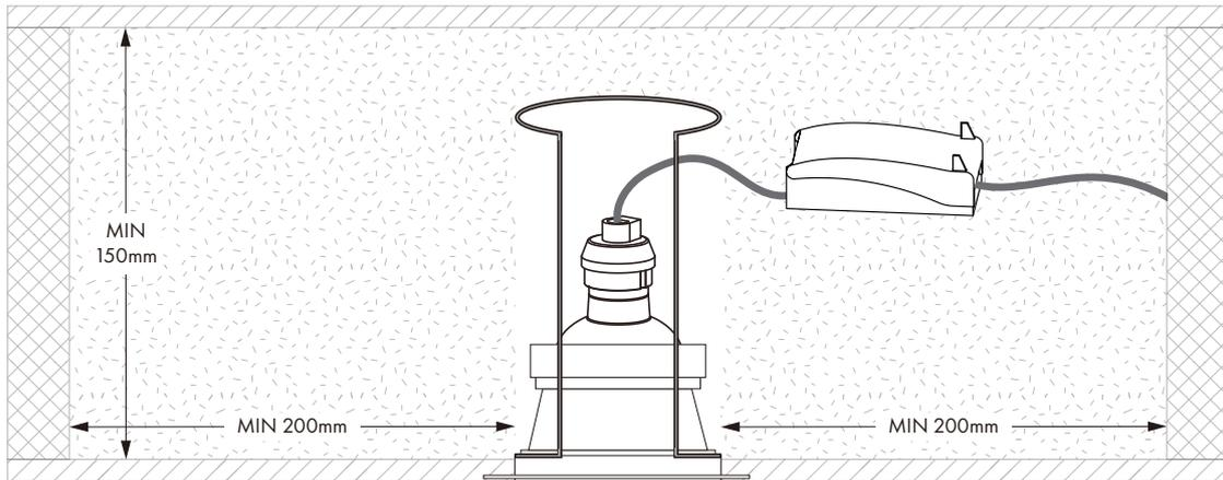
If installing without an insulation bracket please ensure any insulation is at a minimum distance of 150mm away from the fixture / lamp and not covering it.
