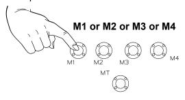
1- Press and hold down one of the push-button **M1 o M2 o M3 o M4** of the receiver, the buzzer will make a beep each time and then sound continuously.
