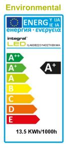
Energy Rating: A+ Lowest Operating Temperature: -20 degrees Maximum Operating Temperature: 40 degrees IP (Ingress Protection) Rating: IP20 Hg 0% (Mercury Free): Yes
