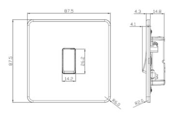
An intermediate switch is used when you have three switches controlling one light. A typical example of this is on a landing. There is a switch at the bottom of the stairs, one at top of the stairs and one at the end of the landing. On this circuit you would need the middle switch to be intermediate (i.e. the one at the top of the stairs) in order for all the switches to function properly
