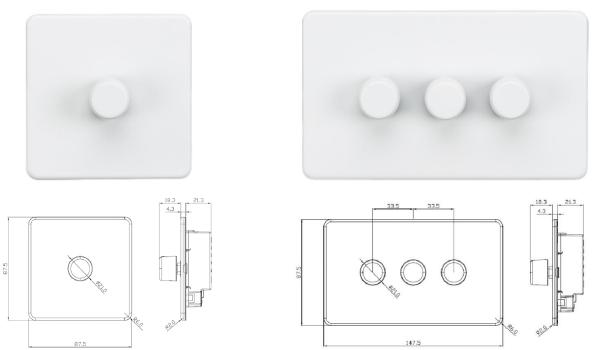
Push on/push off control. Advanced trailing edge type dimmer suitable for dimming all types of lamps both resistive and inductive. Minimum capacity: 5W dimmable LED or 10W incandescent. Maximum capacity: 150W dimmable LED or 200W incandescent. Suitable for mains lighting, low voltage lighting and LED lighting (for compatibility please check with lamp manufacturer.
