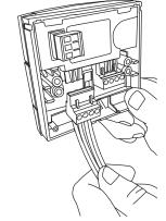
After wiring the terminal connector, plug into the appropriate position, see connection details (left).
