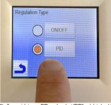
If you wish to use PID mode select "PID" red dot should be lit as in above picture otherwise return to main screen by pressing the return 5 times.
