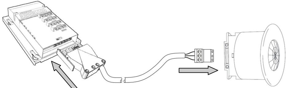
Detector lead supplied with detector.
