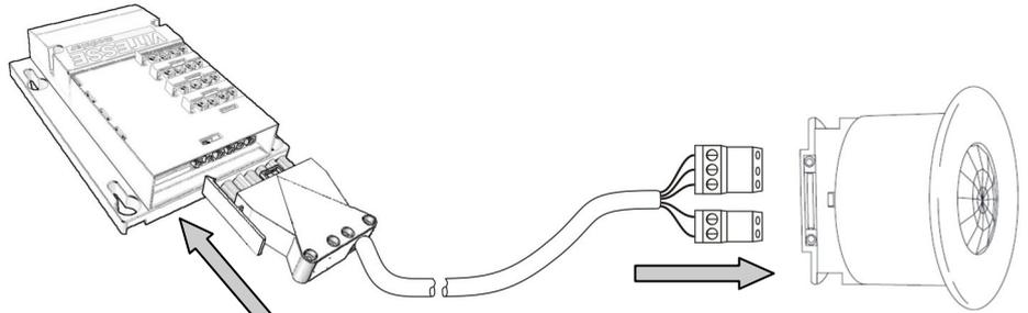
Detector lead supplied with detector.
