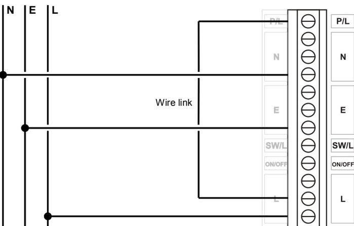
A local lighting switch may still be used when there is a central emergency test switch or when a circuit breaker is used to interrupt the power.
