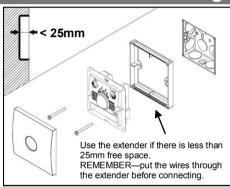
The detector should be sited so that the occupants of the room fall inside the detection pattern shown below, at a recommended height of 1.2m to 1.5m for wall sensors. Note that the higher the sensor is installed the shorter the detection range will be.
