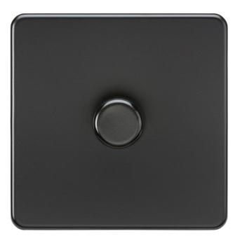
Push on/push off control. Advanced trailing edge type dimmer suitable for dimming all types of lamps both resistive and inductive. Minimum capacity: 5W dimmable LED or 10W incandescence. Maximum capacity: 150W dimmable LED or 200W incandescence. Suitable for mains lighting, low voltage lighting and LED lighting (for compatibility please check with lamp manufacturer)
