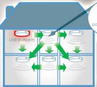
Sianal is received. transmitted and re-transmitted to achieve multiple paths to ensure secure communication
