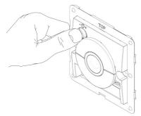
Time setting (determined by switch, see below) 5 sec—15min 15min—2hour
