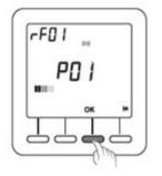
Press and hold the 2nd button from the left for 5 seconds until **tAP** is displayed.
