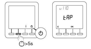
Press and release the **OK** button. The thermostat searches for the receivers to associate. The number of receivers found and associated is displayed is the centre P00, P01, P02, etc.
