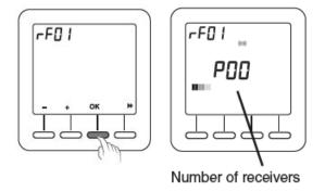
Enter the watts of the unit that the receiver is attached to by pressing the + button. Once finished press the **OK** button. Repeat for every receiver.
