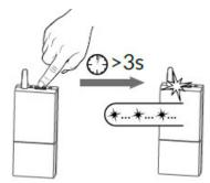
Press and hold the 2nd button from the left for 5 seconds again until rF01 is displayed.
