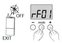
To add more receivers to the same ECRSTAT repeat the above steps. You can add up to 16 receivers to one ECRSTAT. To connect the receivers to the gateway for use with the APP please refer to our gateway guide.
