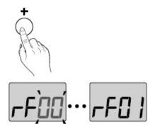
Press and hold the **mode** and **+** buttons on the ECRSTAT simultaneously for 3 seconds or until the display will shows **rF00**.
