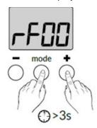
Once the ECAR receiver has paired with the ECRSTAT the receiver LED will stop flashing. You can now exit by pressing the **mode** and **+** buttons simultaneously.
