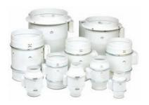
Two-speed domestic axial in-line fans designed to solve ventilation problems for ducted systems. The range is available in six sizes ranging from 100mm-315mm ducting and with airflow performances up to  $1860 \, \text{m}^3\text{/h}$ . Flexible location enables the TD-MIXVENT fans to be connected to any point on the ventilation duct; at the beginning, in-between or at the end, without the loss of any performance.
