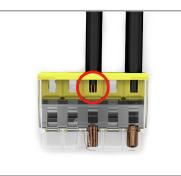
The transparent housing shows if conductors are fully inserted; within the colored base, a clear port shows if the conductor's strip length is correct. Conductors are correctly stripped if the clear port shows no bare conductor on the unprinted connector side. Picture shows center conductor with exceeded strip length.
